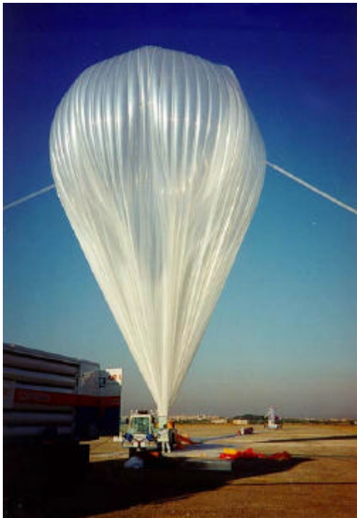
Figure 1 - ARD Recovery System Test Balloon Prior to Launch
