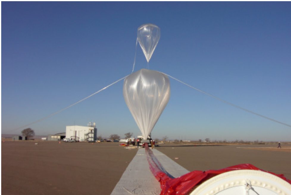
Figure 2 - ULDB Inflation aided by an auxiliary tow balloon attached to the apex fitting
